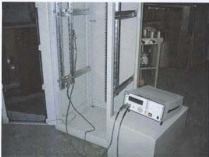
ground continuity between the chassis and the side panel
